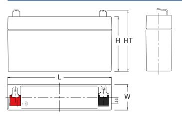
**W**: 0.94 (24) **L:** 3.81 (97) **H**: 2.02 (51.5) **HT**: 2.26 (57.5) Tolerances are +/- 0.04 in. (+/- 1mm) and +/- 0.08 in. (+/- 2mm) for height dimensions. All data subject to change without notice.
