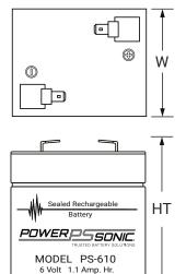
2.00 (51) W: 1.65 (42) 2.00 (51) H: HT: 2.20 (56) Tolerances are +/- 0.04 in (+/- 1mm) and +/- 0.08 in. (+/- 2mm) for height dimensions. All data subject to change without notice.
